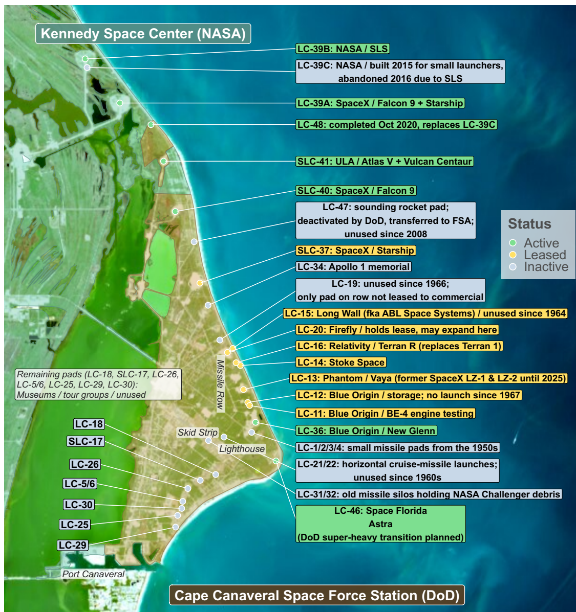
Figure 4.2. Summary of the pads located at the Cape. Map based on Copernicus Sentinel data. Pad locations approximate. Source: Rational Futures compilation from Copernicus Sentinel-2 imagery (2026-03-10), FAA licenses, OpenStreetMap (ODbL), CCSFS/KSC lease records, and public reporting.
