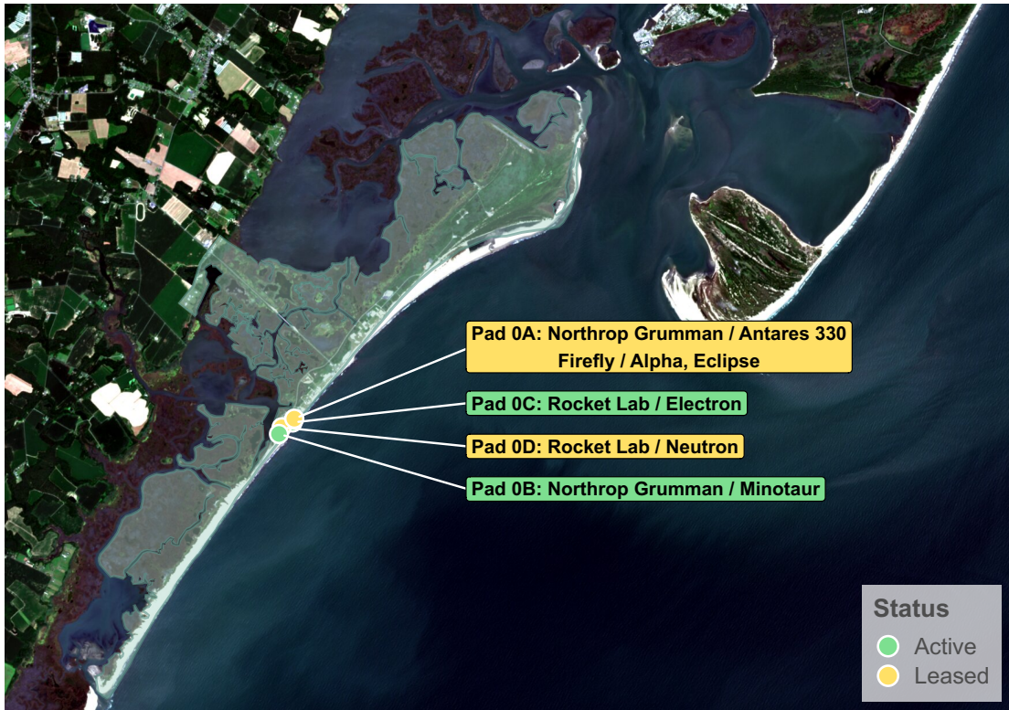
Figure 4.4. Summary of the pads located at the Mid-Atlantic Regional Spaceport at NASA Wallops Flight Facility. Map based on Copernicus Sentinel data. Pad locations approximate. Source: Rational Futures Compilation from Copernicus Sentinel-2 imagery (2025-07-25), FAA licenses, OpenStreetMap (ODbL), NASA WFF and USACE records, and public reporting.
